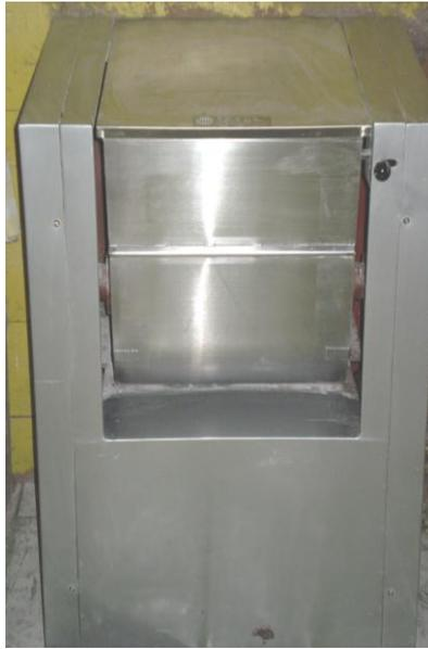
**Figure 4.** Machine for mixing the mixture to form dough before flatten into cakes.
