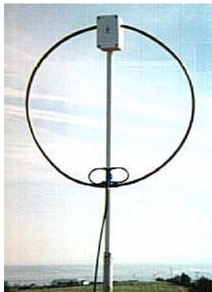
Figure 2.17 Magnetic Loop Antenna [17]
