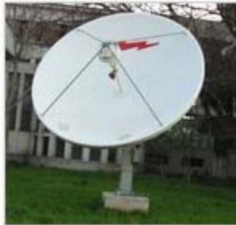
Figure 2.24 Parabolic Dish Antenna [21]
