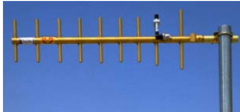
Figure 2.13 A Typical Multiple Elements Yagi Antenna [15]
