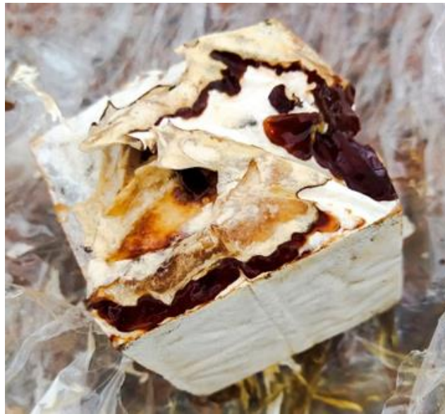
Figure 3.2: Well colonised rubberwood block after 60 days of incubation
