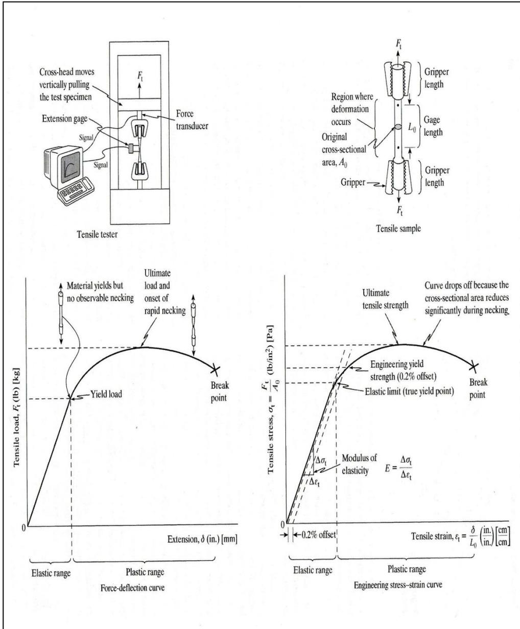
Figure 2.2: Tensile test method and resultant data. [3]
