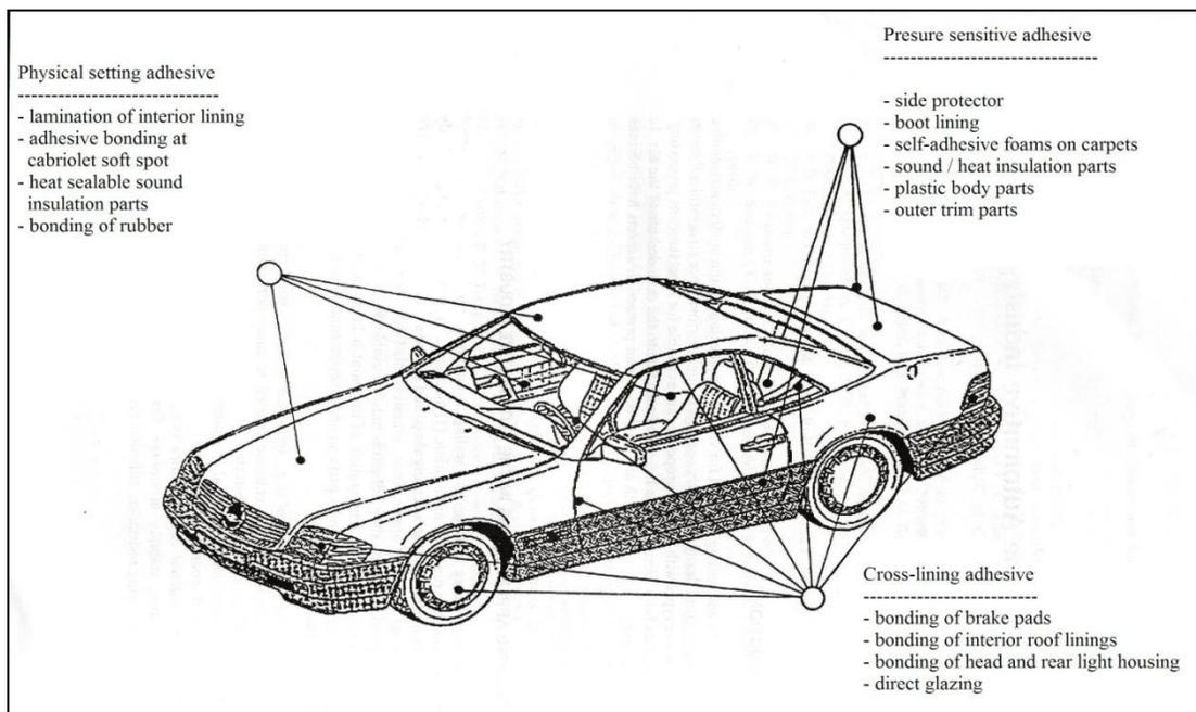
Figure 1.0: Adhesive bonding application in automobile industries [1]
