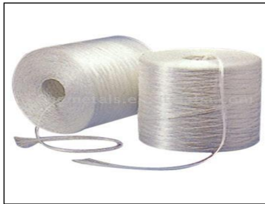
Figure 2.2: E-Glass Fiberglass Roving [6]
