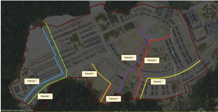
Fig. 7 Completed drainage layout of Taman Uni-Central
