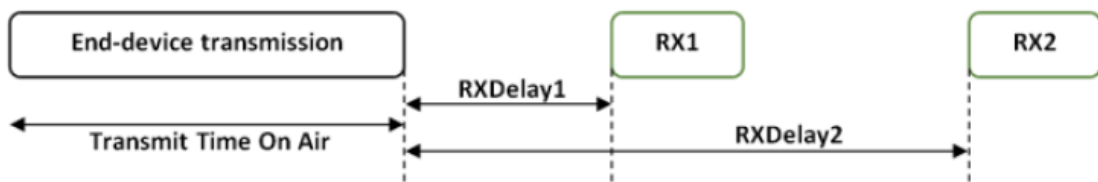
Figure 2.4: Class A LoRaWAN bidirectional communication [11]
