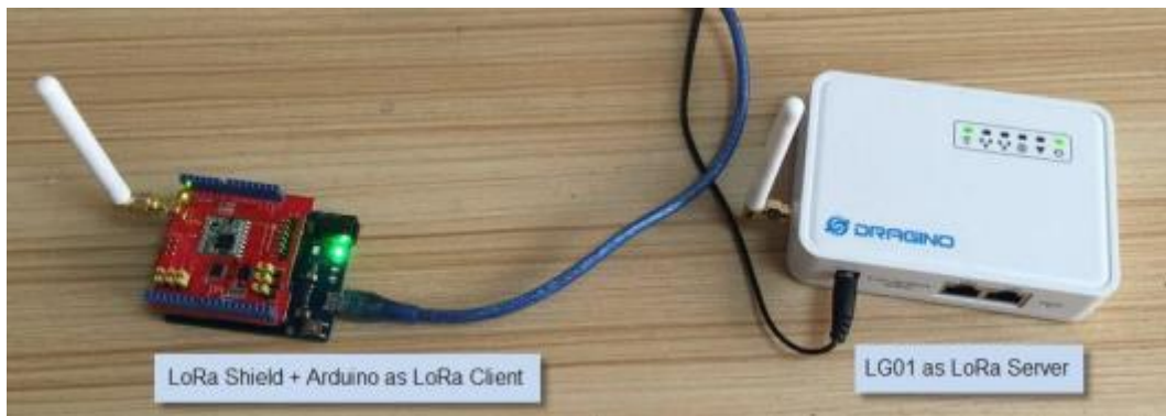
27Figure 4.2: Connecting HMS Device to LoRa Gateway
