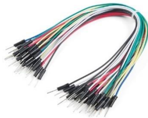
18Figure 3.12: Jumper Wires
