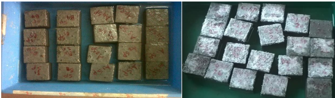
Figure 7 Salt scaling on samples surface before and after Na 2 SO 4 immersion
