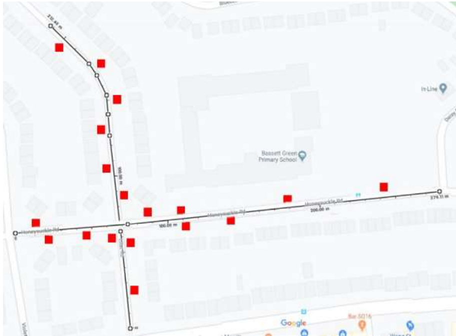
Figure 4.6: The cross-junction road segment with distance of approximately 492 m is simulated in StreetlightSim as cross-junction network topology associated with 19 red dots to represent the streetlights across the residential area (the map was modified from Google Maps).
