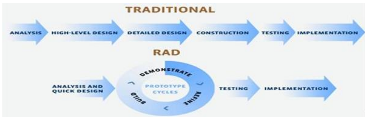
Figure 1.2 the structure of the traditional model and the RAD model
