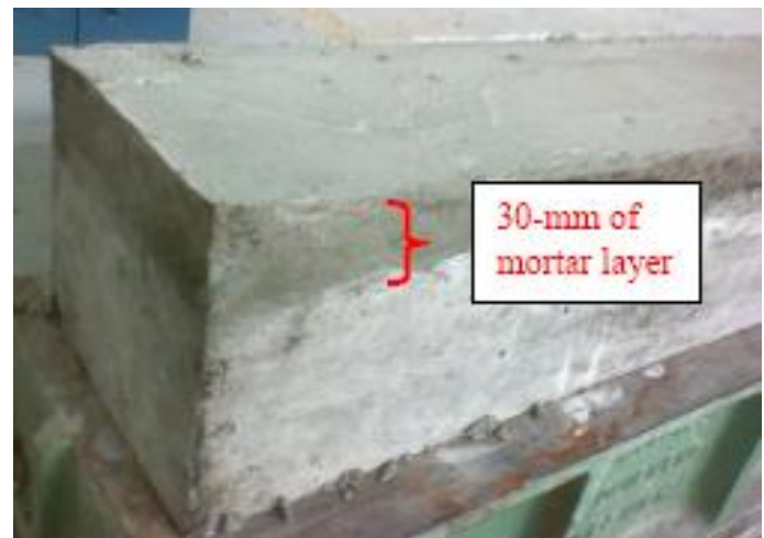
Figure 2: Ferrocement laminate attached to beam.
