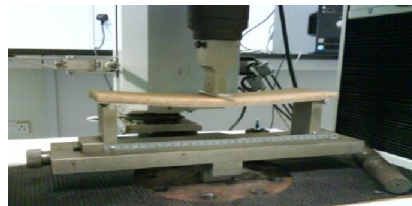
Figure 3: Three point bending test using Testometric machine
