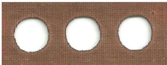
Fig. 9 - Sample holes drilled by diode laser
