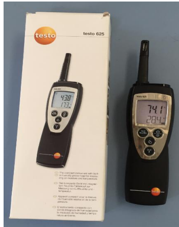
Figure 3.2: Hygrometer Model Testo 625
