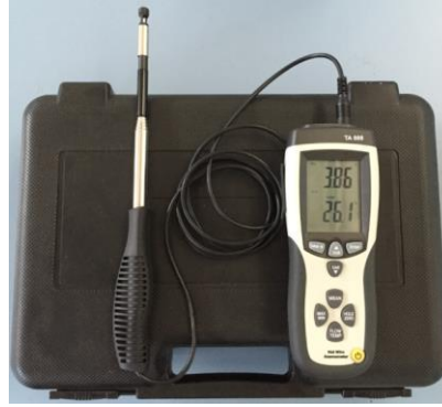
Figure 3.3: Hot Wire Anemometer Model TA 888
