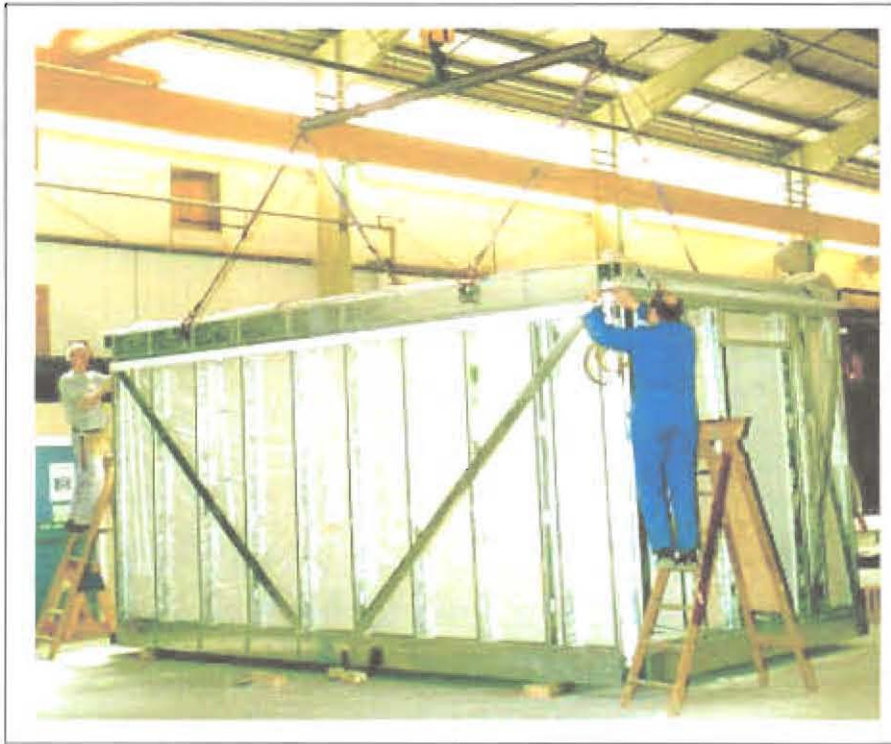
Figure 1.2 A building unit or modular unit formed by cold-formed Steel Members (Source: Corusgroup 2003)
