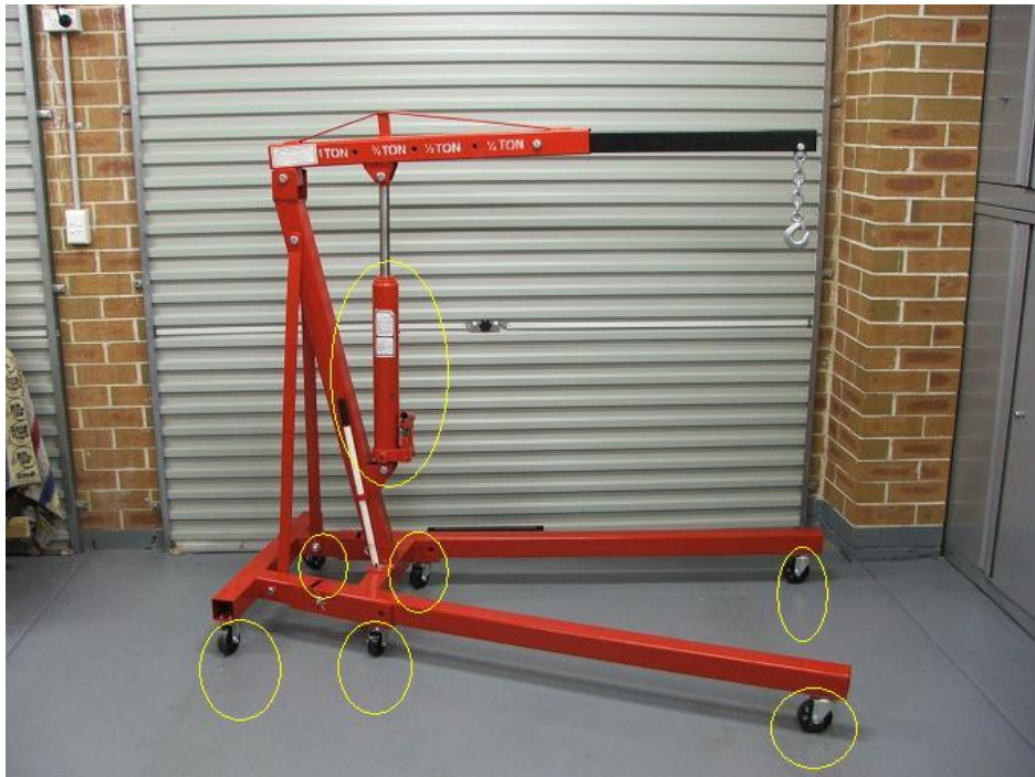
Figure 1.2 The Existing Portable Crane
