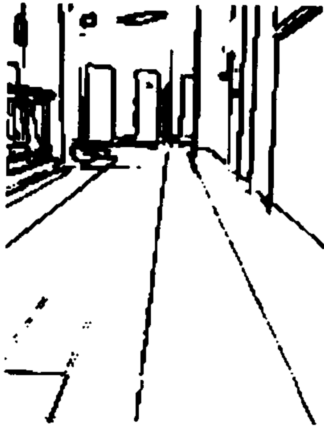
Figure 3c – Output image of Sobel edge detector
