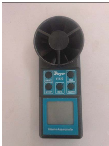
Figure 3.20: Dwyer VT120 integral vane thermo anemometer
