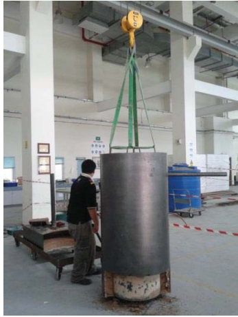
Figure L 47: Pyrolysis chamber is lifted up by overhead crane for transportation
