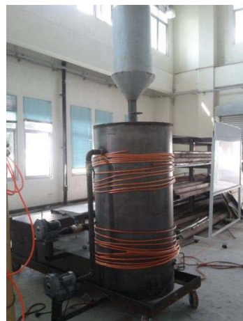
Figure L 70: Copper tubes is surrounded the pyrolysis chamber
