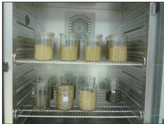
Figure 3.18: Binder drying oven with natural convection
