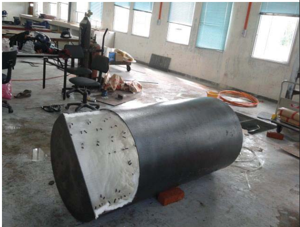
Figure L 19: Side view of the pyrolysis that filled with 12.5-mm ceramic fire blanket
