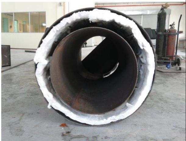
Figure L 21: Filled in pyrolysis chamber (left)
