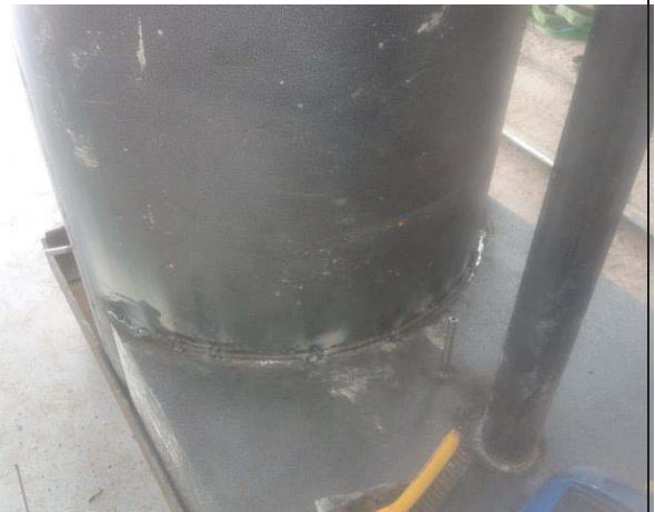
Figure L 50: Welded pyrolysis chamber with tar removal chamber
