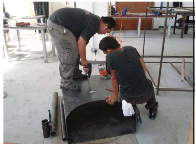
Figure L 10: Drilling thermocouple hole in the tar removal chamber
