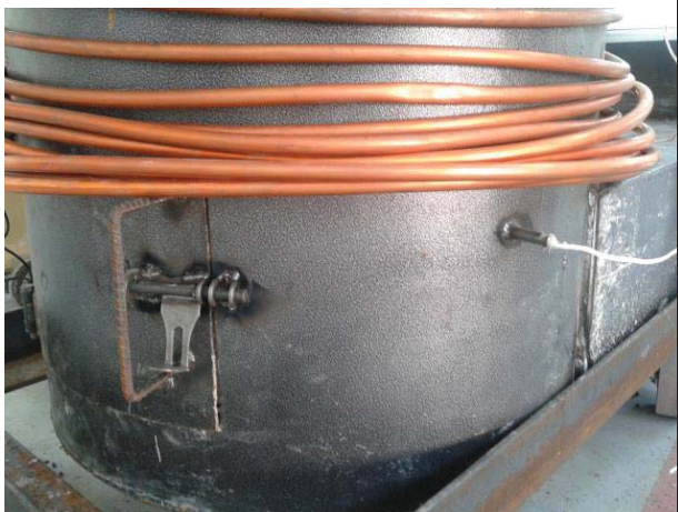
Figure L 69: Door latch is installed at pyrolysis chamber
