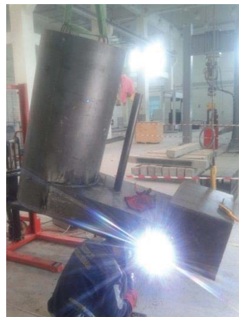
Figure L 52: Welding the fuel gas-to-heat energy conversion chamber with the main body
