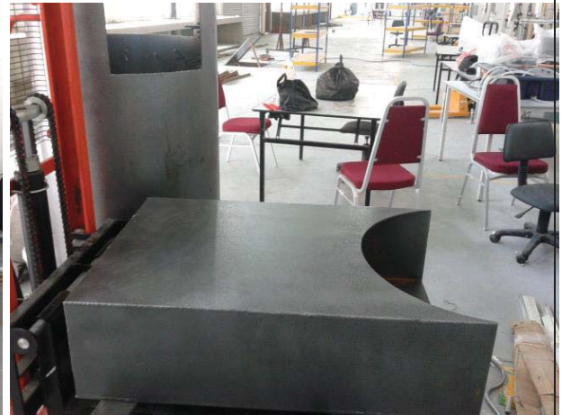
Figure L 8: Galvanized tar removal chamber
