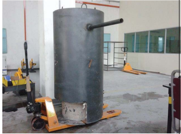
Figure L 48: Pyrolysis chamber is transported back to workshop with a mechanical lifter
