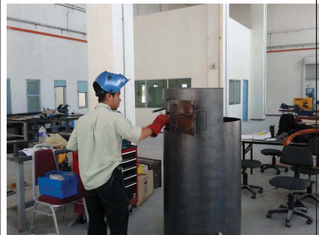
Figure L 16: "V" anchor bar is welded in pyrolysis chamber door
