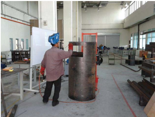
Figure L 3: Cleaning the welded residue
