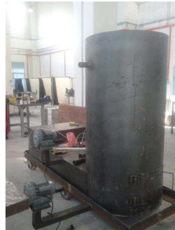
Figure L 56: Blowers is installed on its stand
