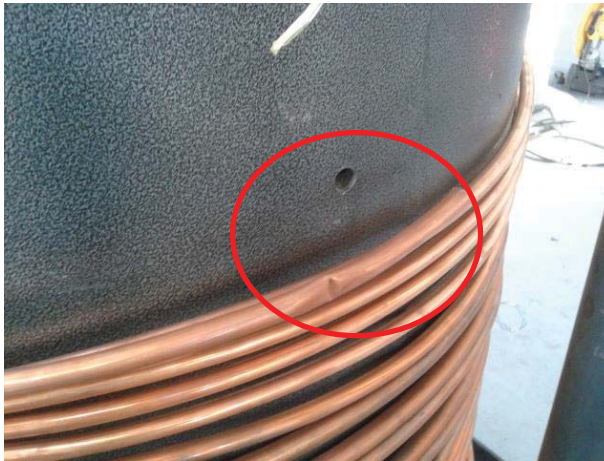
Figure L 73: Discover the difficulty in fit in the copper hole inlet
