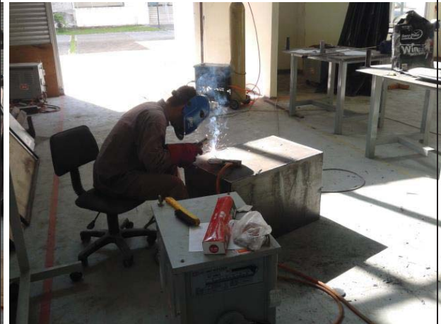
Figure L 14: Welding the fuel gas-to-heat energy conversion chamber
