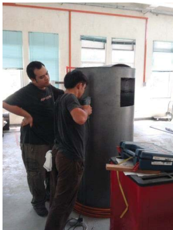
Figure L 9: Drilling thermocouple hole in the pyrolysis chamber
