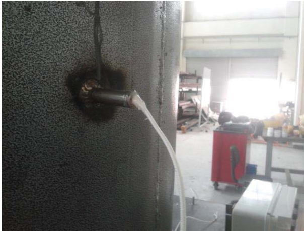
Figure L 59: Installation of thermocouples
