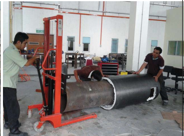
Figure L 20: Fitting the pyrolysis chamber framework into pyrolysis chamber before fill in refractory
