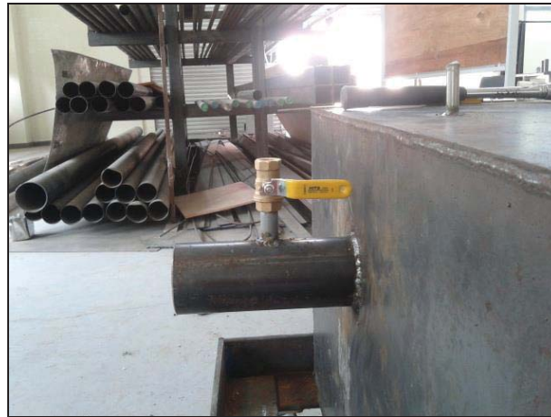
Figure 3.22: Gas sampling probe located in the middle of B2H exhaust
