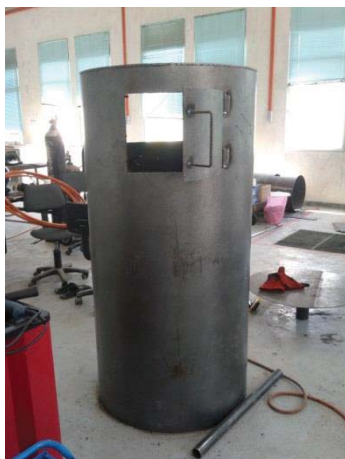
Figure L 15: Pyrolysis chamber door is cut
