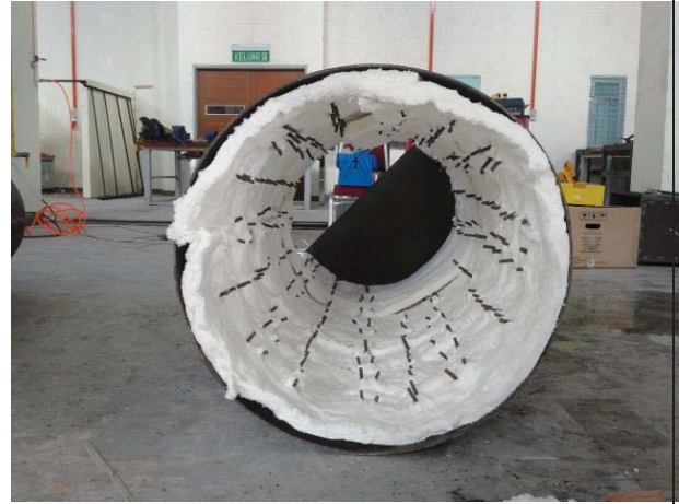
Figure L 18: 12.5-mm ceramic fire blanket is installed inside the pyrolysis chamber
