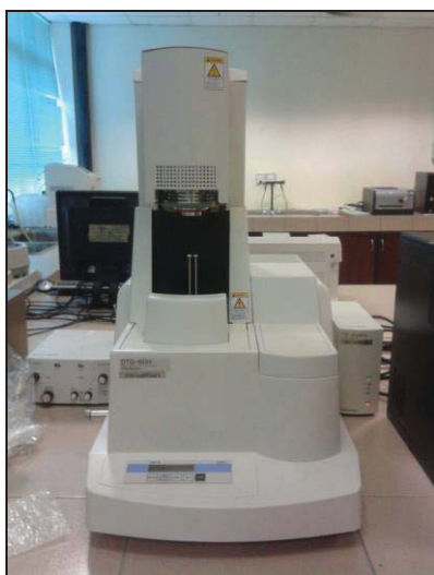
Figure 3.17: Shimadzu DTG-60H thermal analyser
