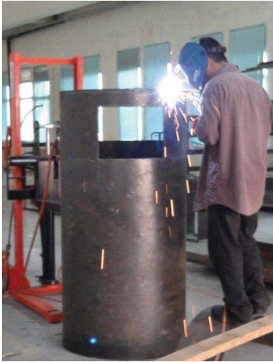
Figure L 1: Welding the base of pyrolysis from outside
