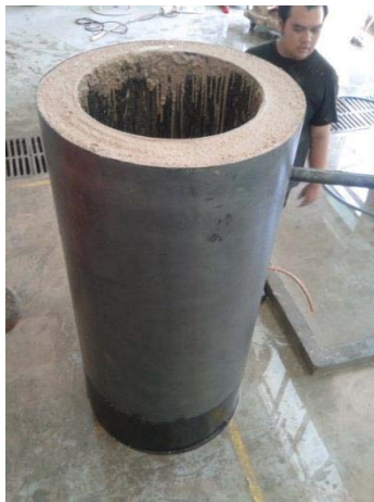
Figure L 39: Filled in refractory inside the pyrolysis chamber (left for 24 hours)
