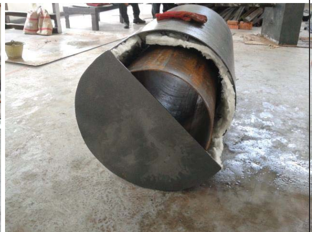
Figure L 22: Filled in pyrolysis chamber (right)
