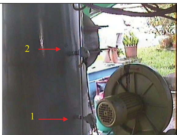
Figure 1.11: Locations of thermocouples 1 & 2
