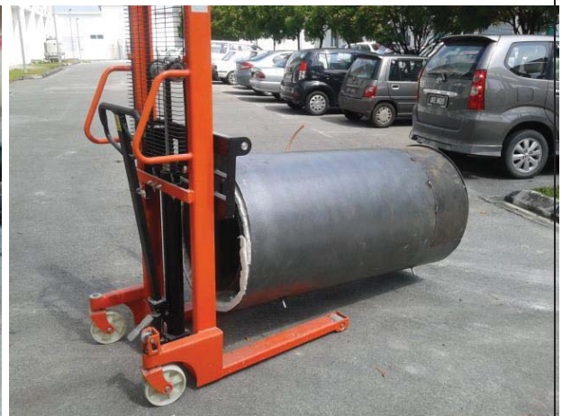
Figure L 32: Pyrolysis chamber is transfer to civil lab by hydraulic lifter
