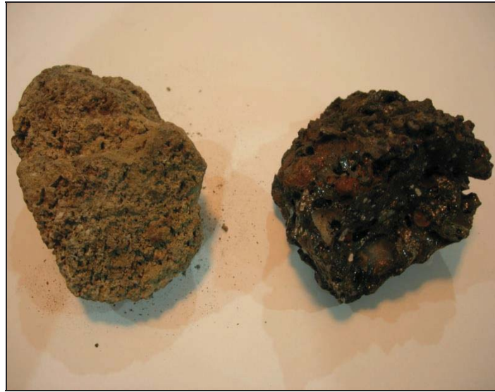
Figure 1.15: Slag formed in pyrolysis chamber
