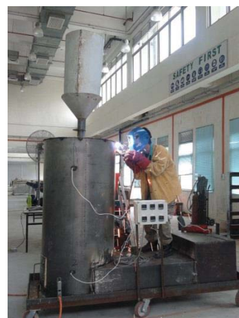
Figure L 64: Welding B2H cover and hopper in the main body
