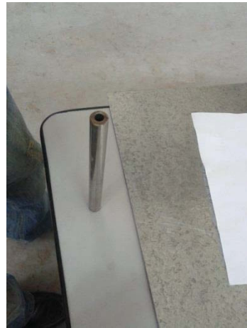
Figure L 12: Lathed stainless steel for use as thermocouple well
