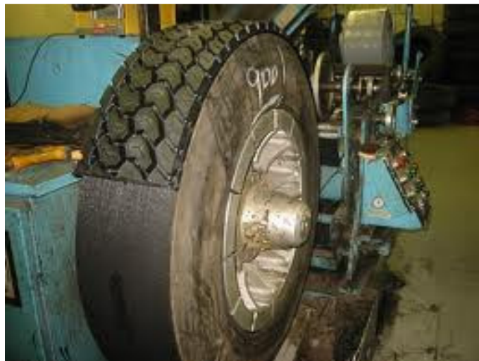
Figure 2.3 – Semi Grinding Process
