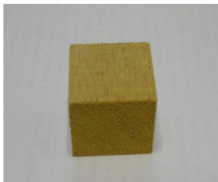
Figure 3.1. Wood cubes (19 mm x 19 mm x 19 mm) for chemical treatment.
