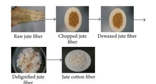
FIGURE 1: Flow chart of the synthesized jute cotton fibers.
