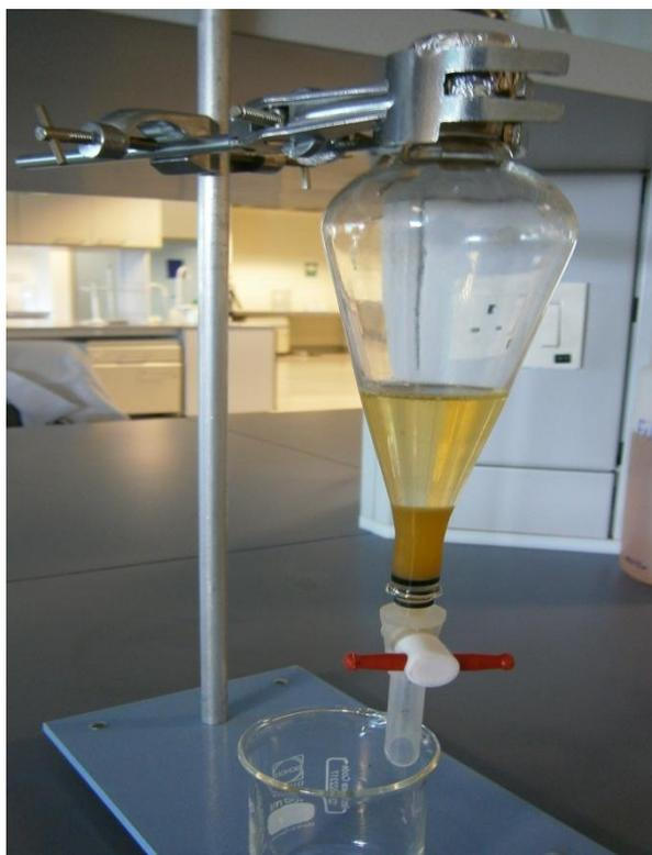
Figure 3: Layers of glycerol and biodiesel
