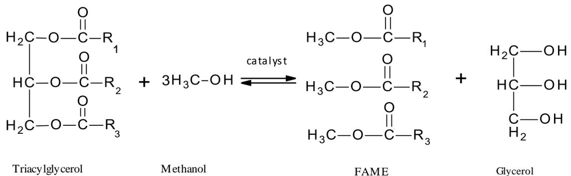
Figure 1: The transesterification process of fatty acid methyl ester (Biodiesel)
