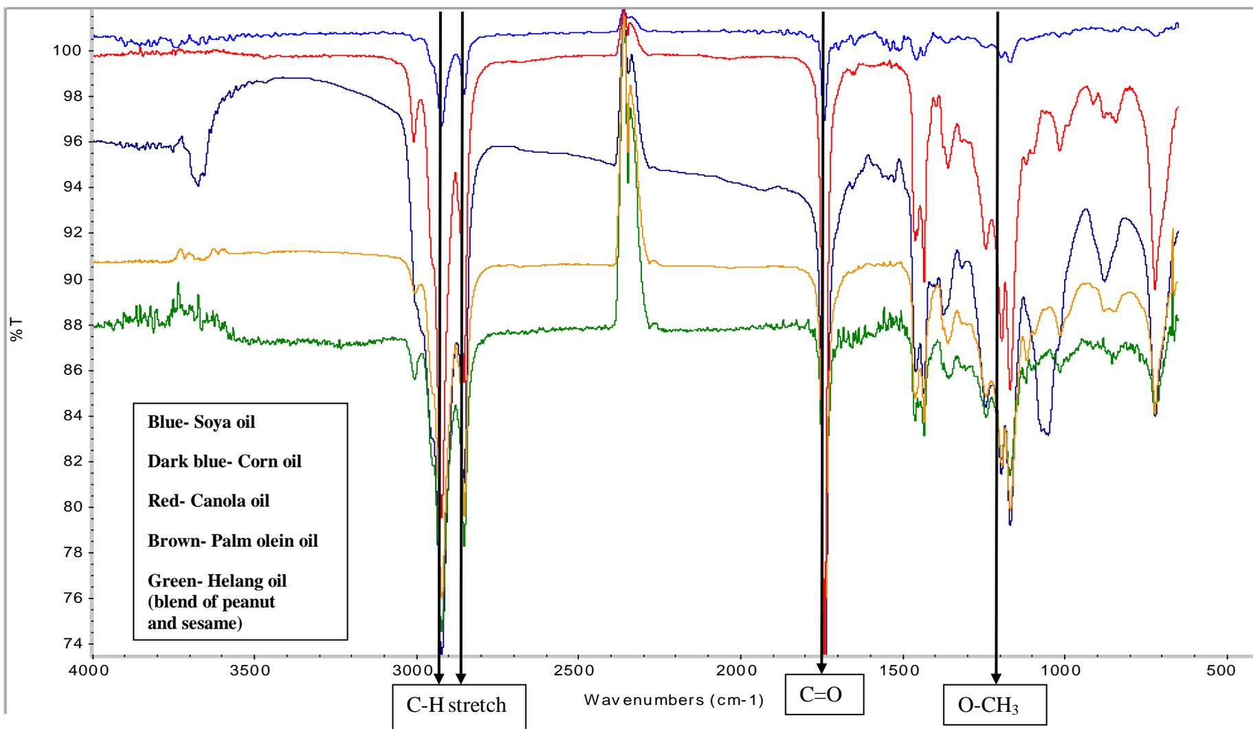
Figure 5: IR spectra of different biodiesels from various origins
