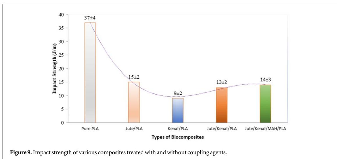
attribute the enhancement in stiffness of the composites to the effect of the coupling agent treatment. MAH coupling agents can modify fiber surfaces to improve jute/kenaf hybrid composites' tensile strength and tensile modulus. The aforementioned attribute makes composites a more suitable choice for applications that require heightened degrees of strength and stiffness [47, 52].
