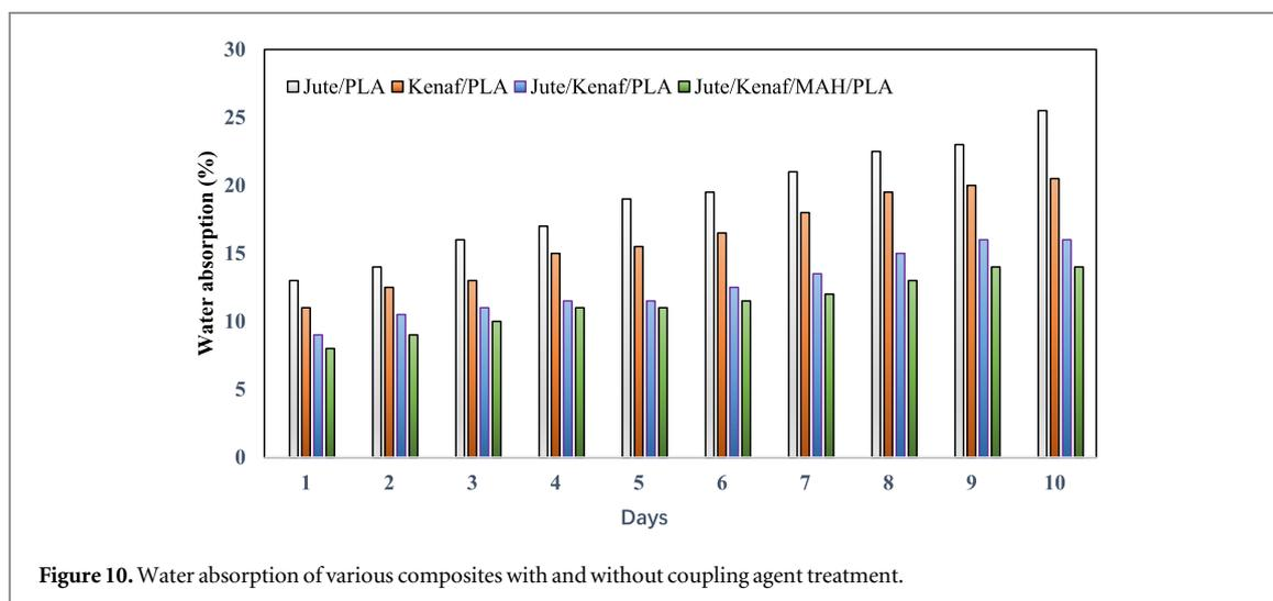
Figure 10. Water absorption of various composites with and without coupling agent treatment.
