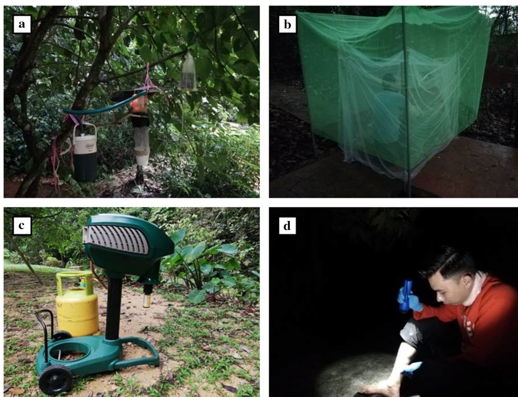
Fig. 2 Trapping methods. a CDC light trap. b Human baited trap (HBT). c Mosquito Magnet (MM). d Human landing catch (HLC)
