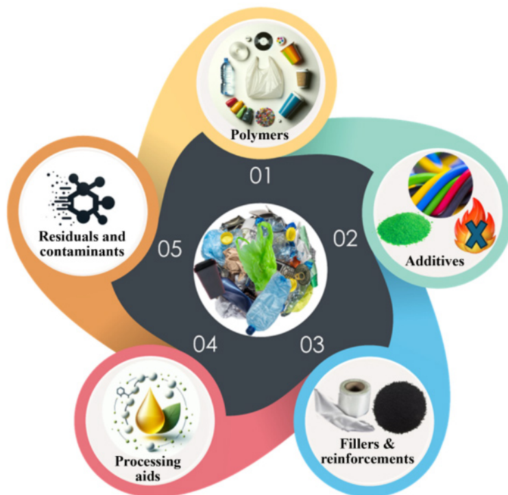
Fig. 1 Plastic waste composition. Plastic waste is composed of a variety of materials, including different types of polymers such as PE, PP, PVC, PET, PS, polycarbonate, PU, PE naphthalate, polytetrafluoroethylene, polyamide, acrylonitrile butadiene styrene, and polymethyl methacrylate (PMMA). Additionally, plastic waste contains various additives like plasticizers, stabilizers, colorants, and flame retardants. Fillers and reinforcements, such as glass fibers, minerals, and carbon black, are also present. Processing aids, including processing oil and lubricants, may be found in plastic waste, as well as residuals and contaminants like residual monomers and other impurities.
