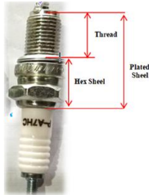
Figure 1. Spark plug layer anatomy.
