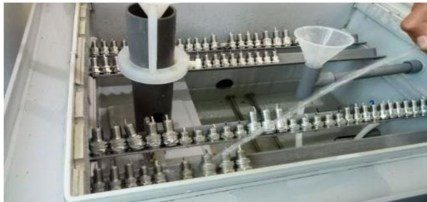
Figure 2. Salt Spray Test process of this study.
