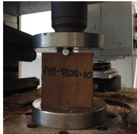
Fig. 4 Embedding strength test setup
