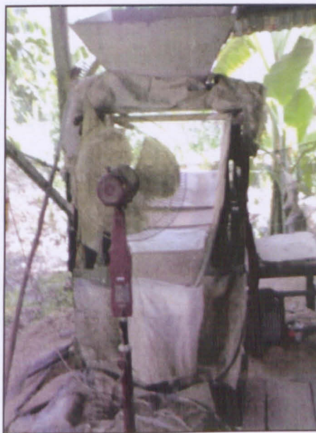
Figure 1.5: The use of fan to remove husk from the rice
