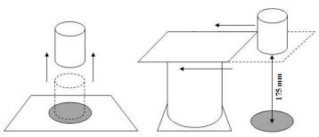
Fig. 1. Schematic diagrams of lift method [left] and drop method [right].
