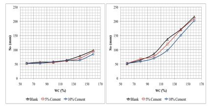
Fig. 2. Flowability test values for lift method [left] and drop method [right].
