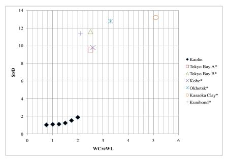
Fig. 3. Normalized results between  $S_D/D$  and  $WC_M/W_L$ .
