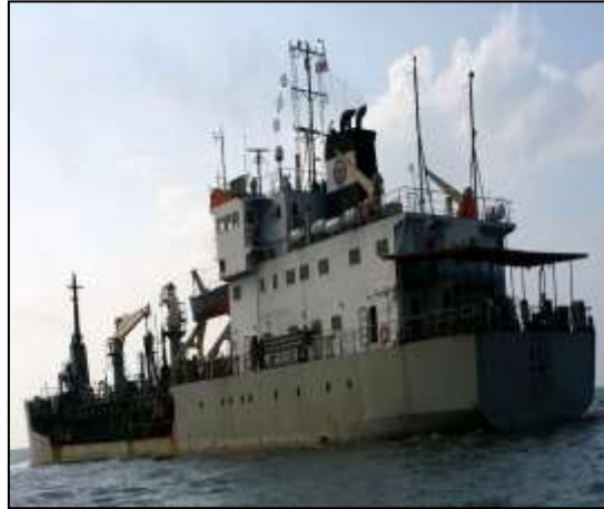
Figure 2. Trailing suction hopper dredger at dredging site (Kuala Muda, Kedah)
