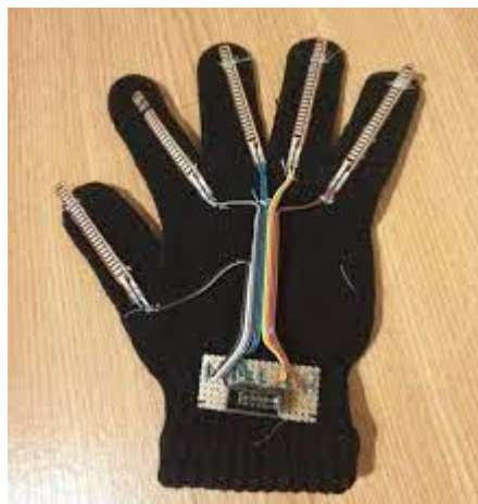
Figure 1: Wearable glove-based sensor approach (Cotoros et al., 2021)
