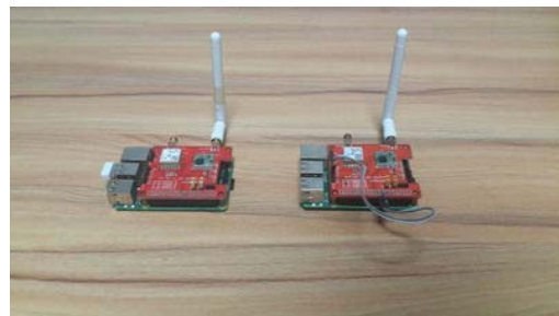
Fig 3. Two Dragino LoRa/GPS shield installed on top of two Raspberry Pi 3
