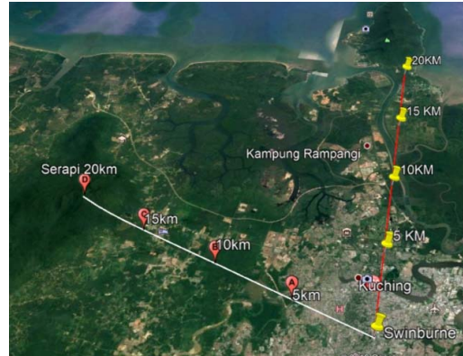
Fig 4. Estimated line-of-sight distance between the location of transmitter and Mount Serapi (white line)
