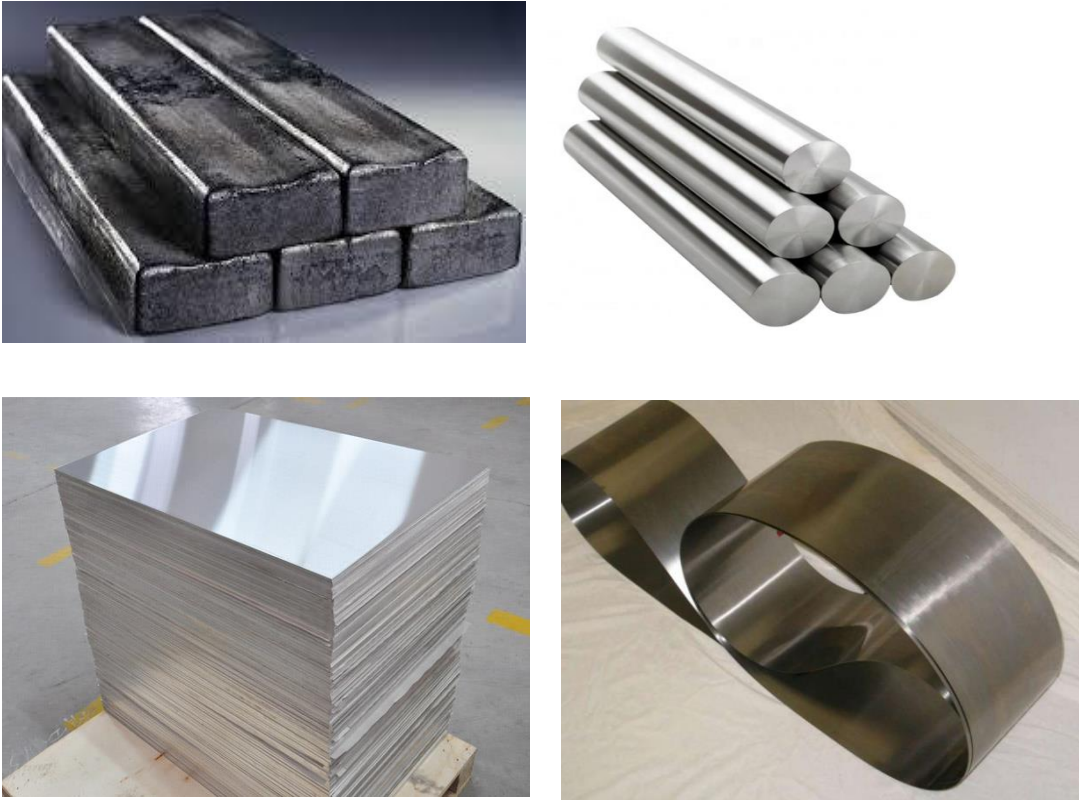
Figure 2.1: Magnesium metals in various forms available commercially. (Courtesy from Press Metal Berhad)
