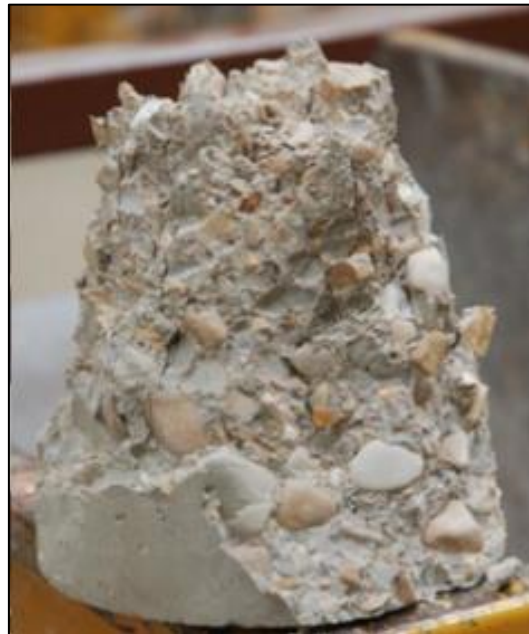
Figure 2.1: Conical rupture of the cylindrical specimen [5]
