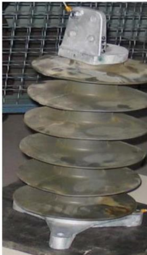
Figure 2.1 A ZnO 20kV Surge Arrester (MOSA) [3]
