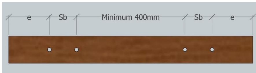
Figure 1.5: Illustration of Timber Bolted Connection Configuration Indicating The End Distance (e), and Bolt Spacing (S b )
