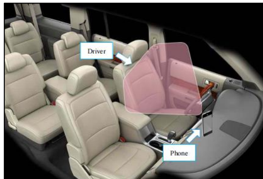
Figure 2.1: Setup of mobile phone in a car for drowsiness detection [13]
