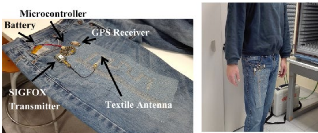
Figure 1.1: Body worn antenna for smart wearable clothing application [2]
