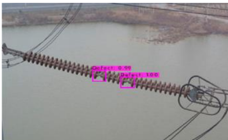
Figure 1.2: Fault detection of insulator using deep learning [6]
