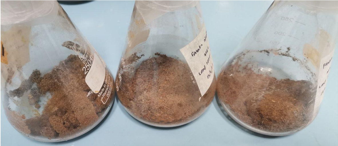
Figure 2.2.1: Erlenmeyer flask that has been inoculated with isolate UMAS MS8 using leaf litter as the substrate in SSF for the optimization of laccase production.
