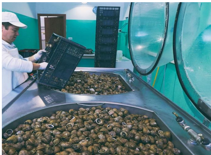
Figure 4: Snails filled into the MullerOne extraction machine (MullerOne, n.d.).
