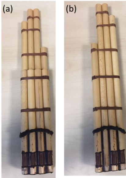
Fig. 4. (a) Tubes 1, 2, 3, and 4 (left to right, length, L = 13\text{cm} ) and (b) Tubes 5, ( L = 19\text{cm} ), 6 ( L = 29\text{cm} ), 7 ( L = 29\text{cm} ), and 8 ( L = 26\text{cm} ) (right to left) with tube no. 7 reed less. All tubes have similar diameter, D=11\text{mm}
