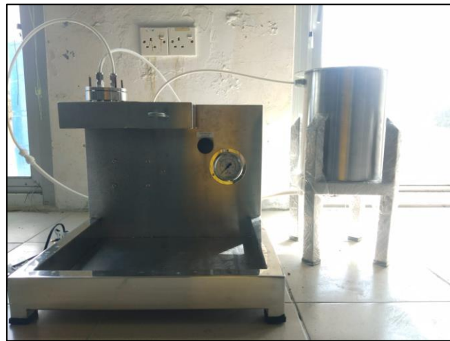
Figure 3.5: Water separation system
