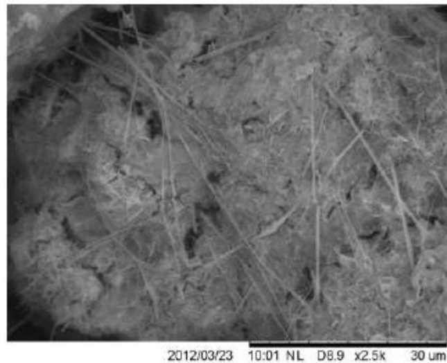
Figure 5: Scanning Electron Microscope (SEM) of mortar with 30% silica fume at w/c 0.4
