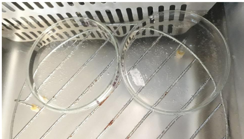
Figure 2: Petri dishes with blank PET sample and incorporated BPA-PET sample put on the water bath.
