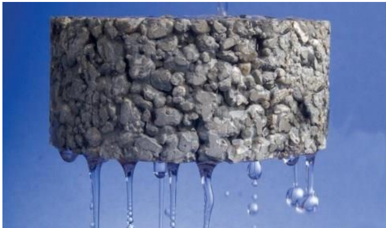
Figure 1: Pervious concrete. (Source: http://www.civilengineeringforum.me/pervious-concrete/ )
