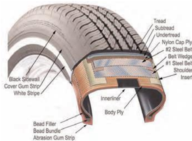
Figure 2.1: Component of Radial Tyre
