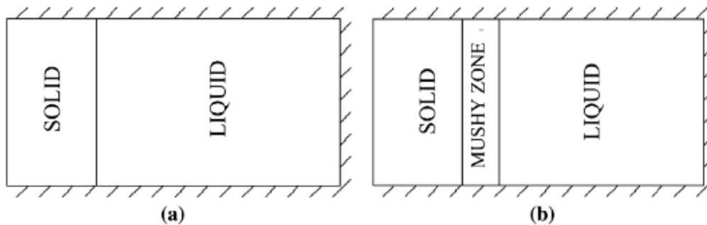
Fig 2.2.1 *solidification scheme (a) pure metal (b) alloys*
