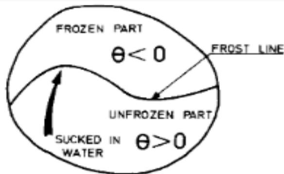
Fig 2.3.1 show that a freezing water saturated soil.
