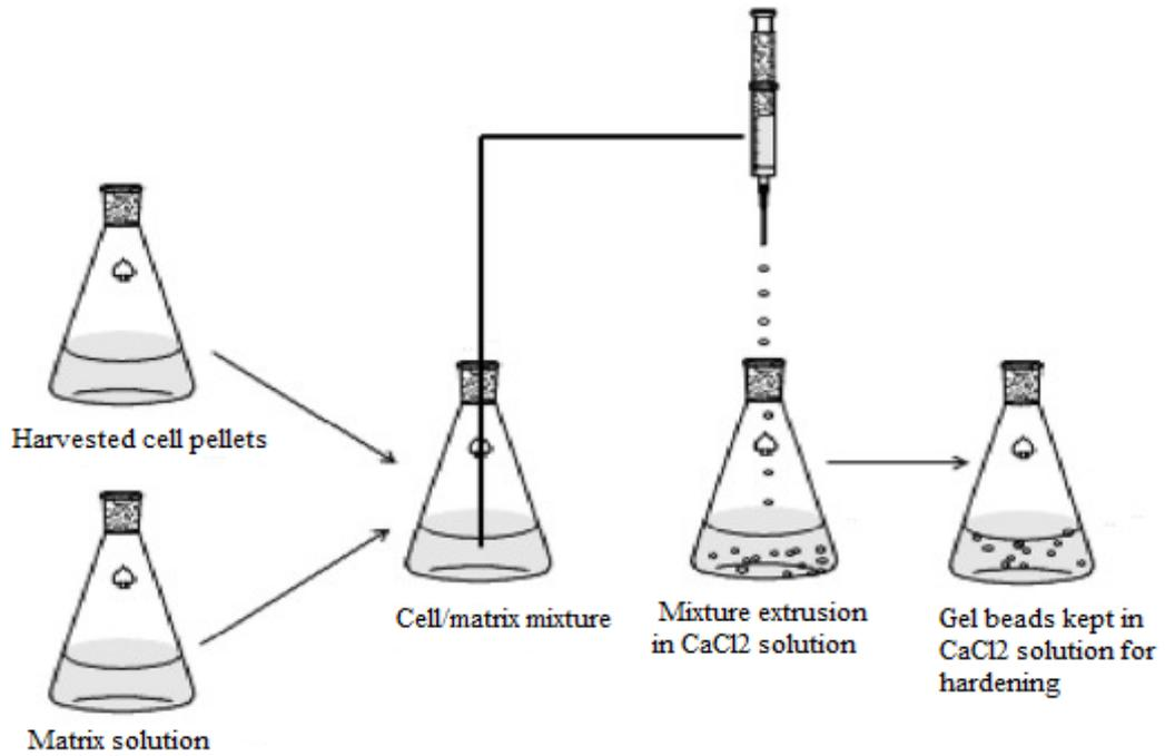
**Figure 3.2:** Schematic diagram for calcium alginate beads production
