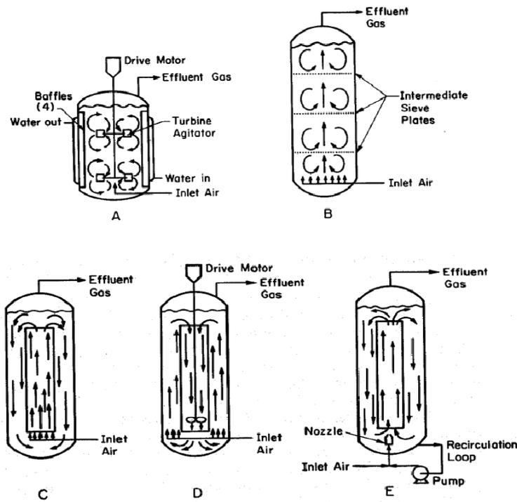
**Figure 2.3:** Bioreactor types; (A) Stirred tank bioreactors, (B) bubble-column bioreactor, (C) airlift bioreactor with central draft tube, (D) propeller loop reactor and (E) jet loop reactor. The arrows in the figure indicates fluid circulation direction
