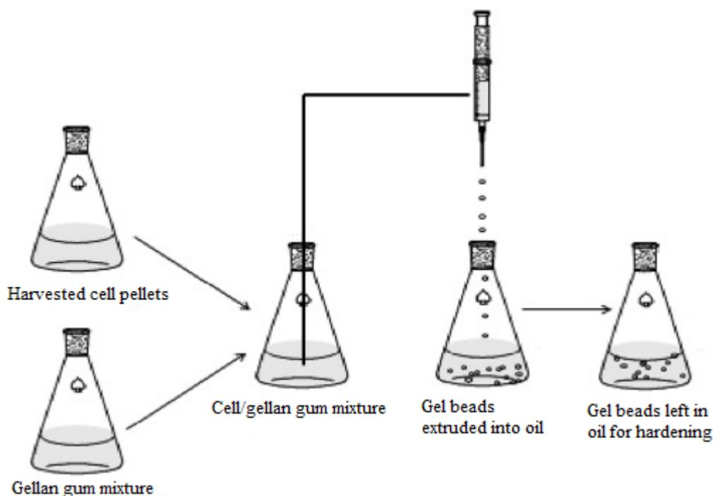
**Figure 3.1:** Schematic diagram of gellan gum beads production
