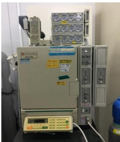
**Figure 3.5:** Gas Chromatography with flame ionization detector (FID) (SHIMADZU GC 14B, Japan)
