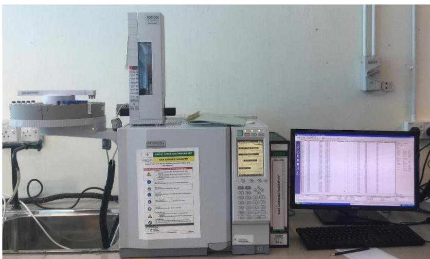
**Figure 5.3:** GC-FID used for the detection of CAR.
