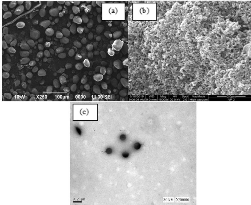
**Figure 3.4:** (a) SEM images of native sago starch, (b) FESEM images of hydroxypropyl starch nanoparticles and (c) TEM images of hydroxypropyl starch nanoparticles
